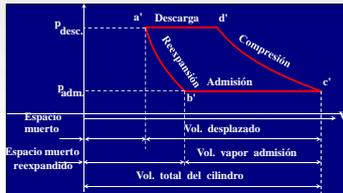
$$V_{b'} = V_{a'} t^{\frac{1}{n}}$$
