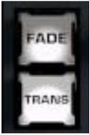
These two buttons provide a quick way to control the *Transition Bin* selection for the delegated switcher layer(s).
