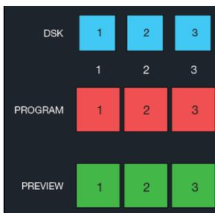
The *first stripe* (nearest the operator) provides three rows of buttons allowing you to choose sources for the various layers comprising TriCaster's primary *Switcher* output.
