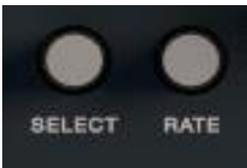
Twist the *SELECT* knob to cycle through the various transition effects that you have added to the software preset bin for the currently delegated video layer. Pressing the knob toggles the *Reverse* option for the current effect.
