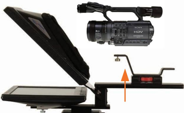
The camera should be mounted with its lens vertically centered in the beamsplitter. Choose the side of the riser that puts the camera in this position. Secure camera to riser with attached camera screw. When camera is mounted slide it gently forward until lens is one inch behind glass beamsplitter. Rotate red knob in "lock" direction to secure camera in place.
