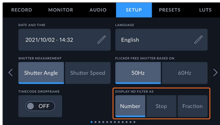
Setup menu in URSA Broadcast G2 with the option to customize how the ND filter information is displayed
