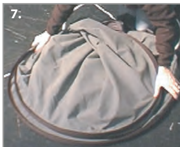
7. Adjust the ChromaFlex frame out evenly towards the edges.
