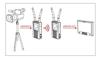
This wireless HD video transmission system uses the latest wireless communication technology and transmits ultra-low latency HD video. The transmitter supports both HDMI and SDI input, while the receiver supports both HDMI and SDI output. It is configurated with OLED display screen and supports iOS & Android App Monitoring.
